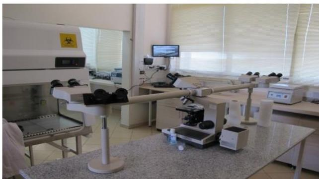
**Figure 3A\_ Five headed microscope**
